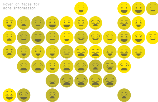
Figure 3: An example of a use of Chernoff-like faces that I actually like, from axios.com [9]. Different health measures for each U.S. state are encoded in semantically relevant facial features. For instance, the size of the bags under the eyes is connected to the percent of citizens who report not getting enough sleep each night.
